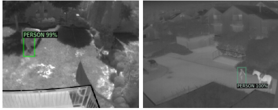
Fig. 9. Examples of Faster R-CNN output images after infrared training.
