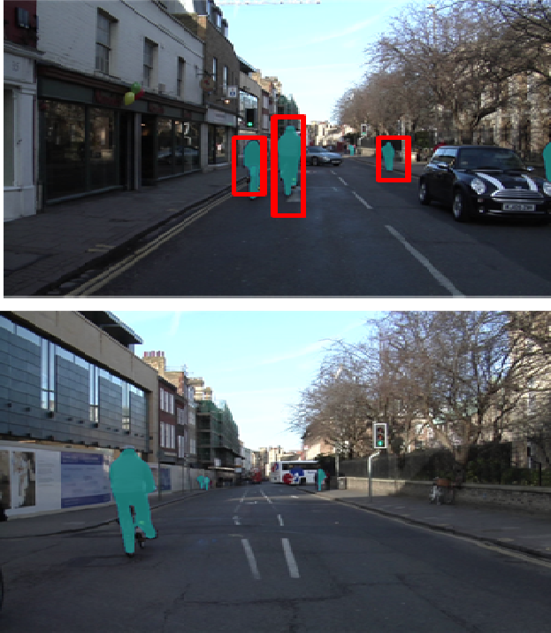
Figure 4: Some instances of the driving scene frames overlaid with segmented salient pedestrian in different configurations (on foot, by bicycle, etc ..). In red, the predicted bounding boxes segmentation.
