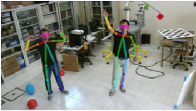
Figure 2: Example of body pose estimation system, a key element of the smart workcell.
