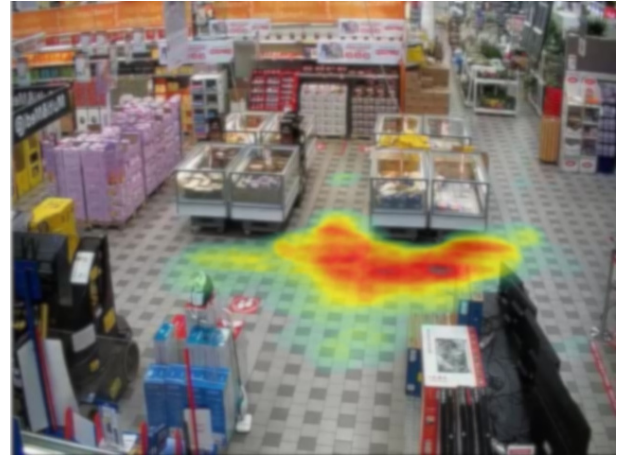
Figure 3: The heatmap in the image represents the areas on which SD violations mostly occur. The heatmap is produced using observations collected in 1-hour from a monitored retail shop. The area with the most observed violations is due to an exhibit placed in the main entrance of the shop that causes increasing SD violations.
